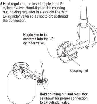
**6.**Turn the coupling nut clockwise and tighten to a full stop. The regulator will seal on the back-check feature in the LP cylinder valve, resulting in some resistance. **An additional one-half to three-quarters turn is required to complete the connection. Tighten by hand only – do not use tools.**
